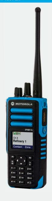
"FROM 1ST JULY 2018, ALL SHIPS ARE REQUIRED TO CARRY A MINIMUM OF TWO PORTABLE TWO-WAY RADIOS FOR FIRE-FIGHTERS, AND DEPENDING ON THE SIZE AND TYPE OF SHIP, THEY MAY NEED MORE. THE RADIOS HAVE TO BE INTRINSICALLY SAFE, AND FOR EU-FLAGGED SHIPS THAT MEANS THEY HAVE TO BE ATEX CERTIFIED."
